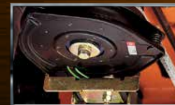
Ogura PTO clutch brake for easy deck engagement. Adjustable internal air-gap for long life.
