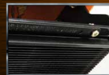
Auxiliary hydraulic oil cooler on the 48", 52" and 61" V-Ride keeps oil temperatures well within a safe operating level and adds to hydraulic system component life.
