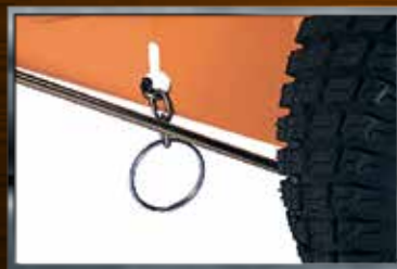
SWZ: De-clutch cold-start feature enhances cold weather starting. It uses a large, easy-to-pull chain that locks into a slot in the engine deck to relieve pump pressure.
