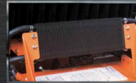
Hydraulic oil coolers and/or pump cooling fans extend component life – Turf Tiger™, Cheetah, Freedom Z®, V-Ride™ and SWZT.
