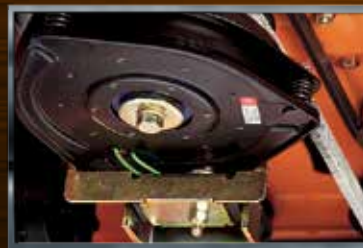
Heavy-duty Ogura GT3.5 clutch features 250 ft/lbs of holding strength. Adjustable air-gap for long life.
