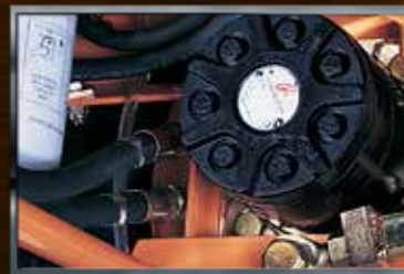
High-torque, cast-iron wheel motors ensure dependability. Heavy-duty drive system is designed for reliability.
