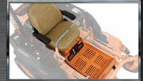
Operator Suspension System with a coil-over shock provides incredible, adjustable comfort without affecting cut quality – Cheetah™.
