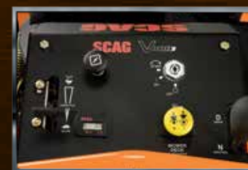
Easy to reach, full-featured instrument panel has ignition key, cutter deck engagement switch, drive and neutral lever, throttle, choke and digital hour meter.
