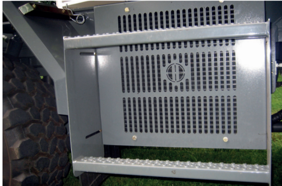
Hydraulikölkühler am Unterwagen // Hydraulic oil cooler mounted to the undercarriage
